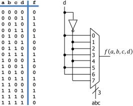
✓ Implement the previous circuit using <u>ONLY</u> 2-to-1 MUXs (AND, OR, NOT, XOR gates are not allowed). (14 pts.)  $f(a, b, c, d) = \bar{a}f(0, b, c, d) + af(1, b, c, d) = \bar{a}(b\oplus(c\oplus d)) + a(\bar{b}\oplus(c\oplus d)) = \bar{a}g(b, c, d) + ah(b, c, d)$
